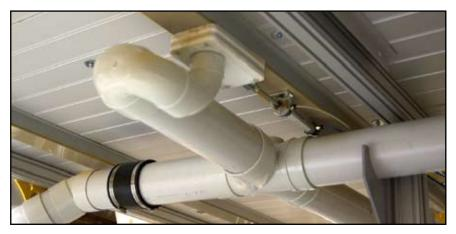
On smaller Aeronaut vacuum tables, the blast gates are normally fitted directly to the collection extrusion and there are normally two per panel. The blast gates can be operated either by hand using a simple rope-pull to open and shock chord to close.
