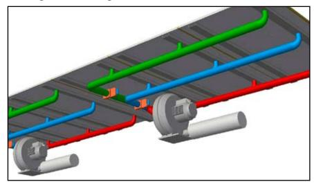
The home side pipe is normally open, and the away side pipe(s) are connected via blast gates to each vacuum pump. The vacuum table is sectioned by the blast gates and switching the pumps themselves.
