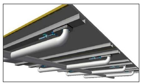
The above picture shows the general layout of a small table fitted with one vacuum pump and pneumatically operated blast gates. The main vacuum pipe runs down the centre line of the table, underneath the table decking.
