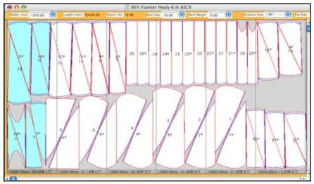
The picture above shows a 75 metre nest for a 12 metre table. The first 8 panels, highlighted, will fit in the first frame. If we select plot across frames, the plotter will plot the entire queue, frame by frame. If we select No plotting across frames, then the plotter will only plot these first 12 frames. The user then pulls the uncut edge of the fabric down to home.
