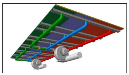
The above illustration shows a vacuum table fitted with two pumps. Each pump connects with several vacuum panels, and each panel is divided width-ways into several cells allowing a wide range of variations to the active vacuum area. The air flow is switched by blast gates (coloured orange) and by the switching the pumps themselves.
