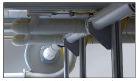
The plumbing is connected directly to the bottom of the collector channels runs via 90° fittings into two or more main tubes running to the vacuum pump. A large blast gate is used to close off these tubes and the plumbing is arranged so that part or all of the vacuum panels to an area of the table can be opened or shut by this blast gate.
