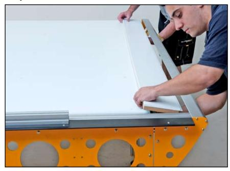
If you do not have enough space to allow for dead zones, the vacuum table can be made without dead zones. In this case you lose about 50 mm from the home end of the table and the parking distance of the plotter (about 450 mm) from the away end of the table. These areas can be masked off so you minimise vacuum "leaks".
